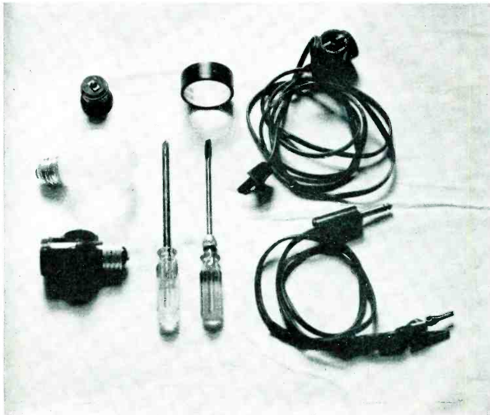
Equipment to take along to drive-in theatre, in addition to your recorder: extension, alligator-clip jack cord for the speaker, roll of electrical tape, regular and Phillips-head screwdriver, socket plug and spare light bulb (just in case you break one belonging to theatre).
